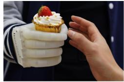
An MIT-developed inflatable robotic hand gives amputees real-time tactile control. The smart hand is soft and elastic, weighs about half a pound, and costs a fraction of comparable prosthetics. Credit: Courtesy of the researchers But this high-tech dexterity comes at a price. Neuroprosthetics can cost tens of thousands of dollars and are built around metal skeletons, with electrical motors that can be heavy and rigid.
