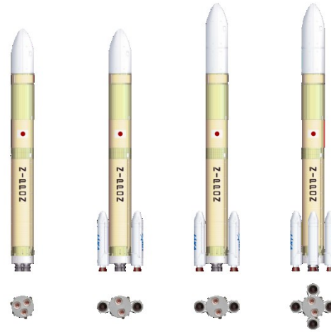
Enlarge / Four configurations of the H3 rocket, with and without boosters, and a larger second stage. JAXA
