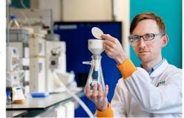
Lech-Gustav Milroy of Eindhoven University of Technology demonstrating the simple paper filter separation method he used to replace expensive HPLC separation. In the background you can see the previously used HPLC equipment. Credit: Bart van Overbeeke/TU Eindhoven.
