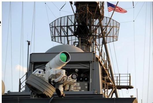
The USS Ponce's laser can shoot down aircraft U.S. Navy photo by John F. Williams/Released
