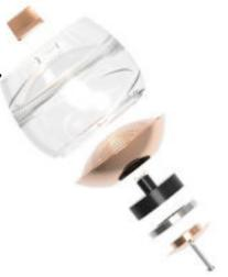
Pieces of a space whisky glass: a gold mouthpiece where a space traveler would sip the whisky and a 3-D printed plastic viewing dome with a helical channel for the whisky to travel up from the convex gold-plated bottom that would hold the reservoir of liquid. The glass would be filled through the black one-way valve on the bottom, and a magnet would allow it to sit firmly to a metal surface. Open Space Agency
