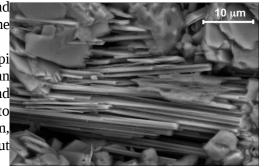
The presence of the mineral actinolite in the caprock of Campi Flegrei provided the crucial clue to unraveling the chemical processes that formed the concrete-like rock beneath the caldera. Courtesy of Tiziana Vanorio
