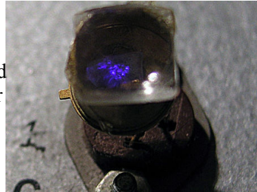
The first blue LED, developed by Maruska.
