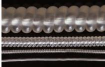
*Fishing line of different diameters, formed into the coiled-coils used in these experiments.* Science/AAAS The researchers found that if they made the fiber form larger coils in the same direction as the initial twists, the fibers contracted. If the fibers were made to coil in the opposite direction from the twist, the fibers expanded. By combining large quantities of these twisted fibers, the team could produce artificial muscles with above-average characteristics.
