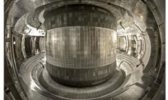
The interior of the donut-shaped Experimental Advanced Superconducting Tokamak (EAST). Hydrogen plasma is confined in this chamber by strong magnetic fields, where it fuses into heavier nuclei. Institute of Plasma Physics, Chinese Institute of Science
