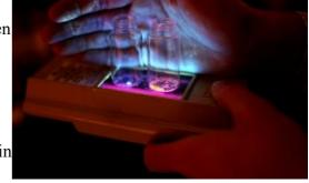
Organic phosphors developed at the University of Michigan could one day lead to cheaper organic light-emitting diodes. Here, they glow in blue and orange when triggered by ultraviolet light. Marcin Szczepanski, U-M College of Engineering
