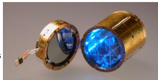
IMAGE: This is the BGO scintillator crystal (right, blue) and germanium disc (left). IAS / SINC
