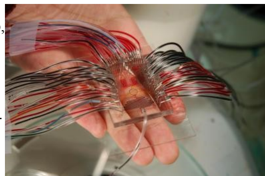
This is a microfluidic device held in the palm of the hand. UCLA
